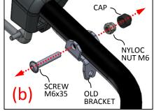
STEP 2: Throw away old cable bracket (a). Then install new cable bracket (b) and reinstall cable (c)
